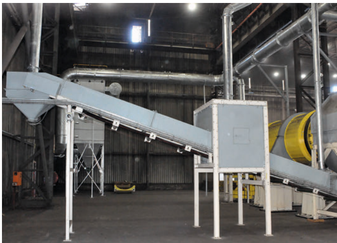
The sand waste, dust and other impurities are removed from the waste material. The new process also offers significant overall environmental benefits through the containment of the cleaning process
