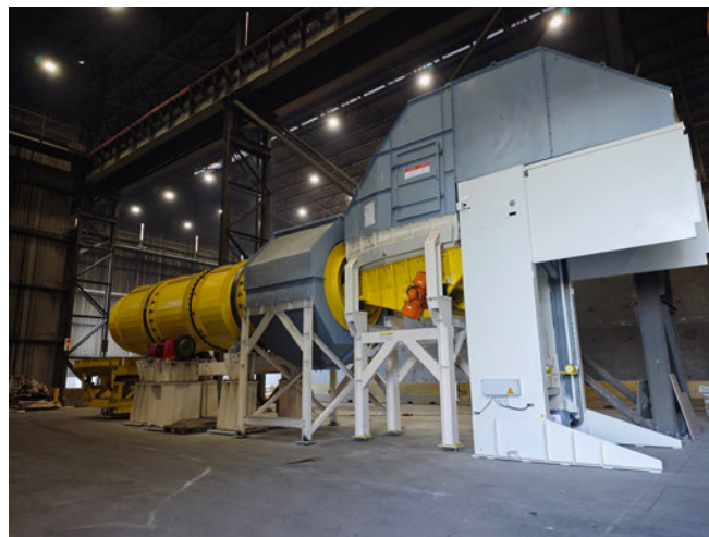
Atlantis Foundries have also invested in a new rotary sprue cleaner drum. The photo was taken during the installation period
