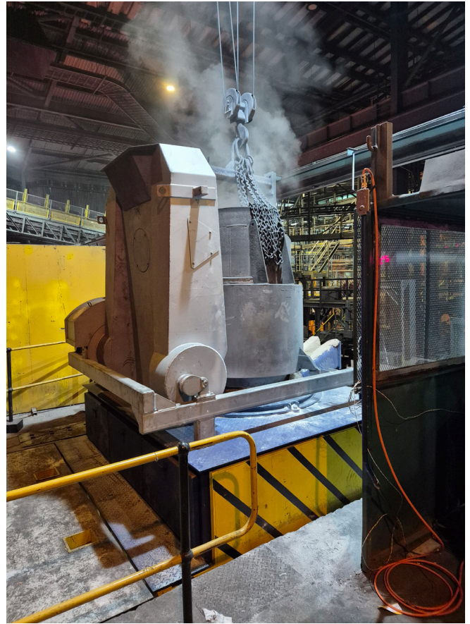
Streamlined furnace charging – powered by charge bucket system
