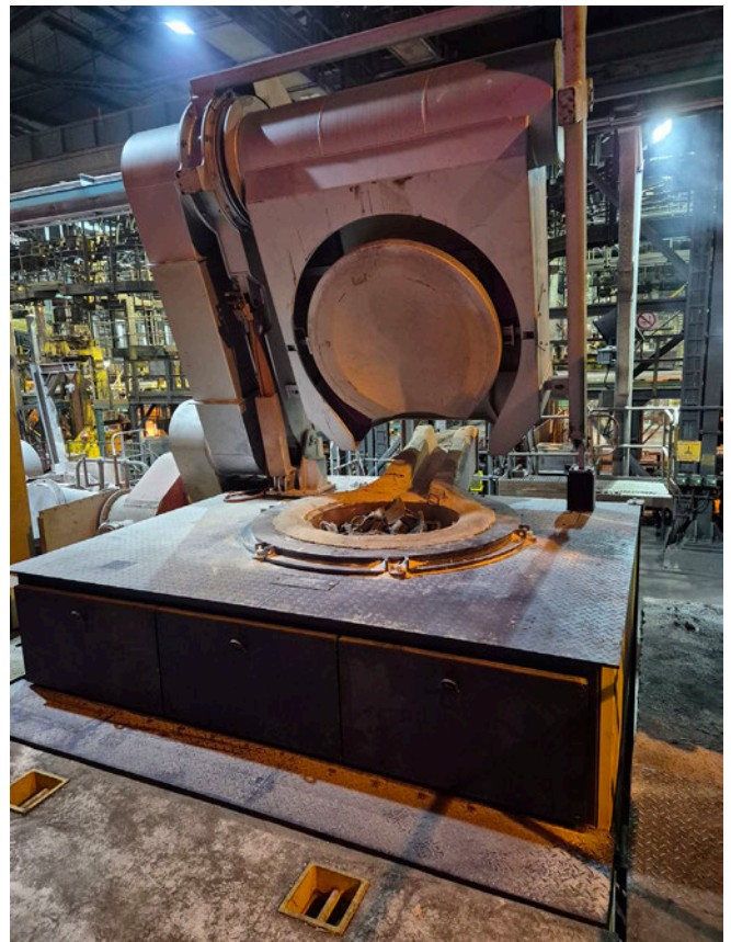
At the South African site, ABP Induction installed an FS40 furnace system using the digital DICU3 unit to control the rectifier and inverter, along with an S7-1500 PLC and 22-inch HMI for furnace operation
